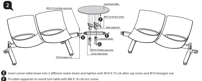
G Slot round turn table + table supporter and u-bracket lower into corner table beam and tighten with M10 X 70 allen cap screw.
