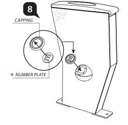
• Insert the \*number plate to the Capping, then insert the assembled parts into the bulb cover.
