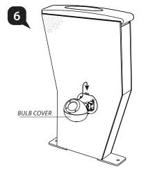
Slot the bulb cover to the steel bracket.
